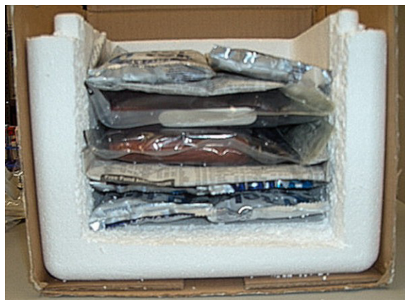
Exhibit 2-2. Packing configuration for two pressure bags
