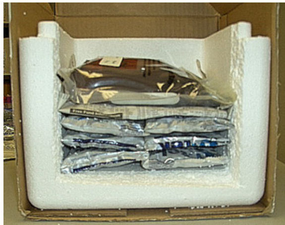
Exhibit 2-2. Packing configuration for two pressure bags
