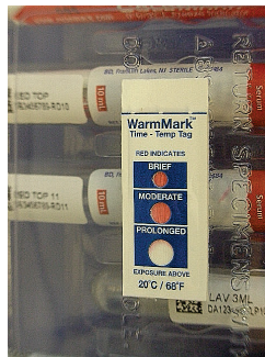
Exhibit 2-14. Triggered upper threshold temperature monitor
