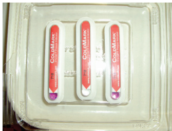
Exhibit 2-15. Lower threshold temperature monitor
