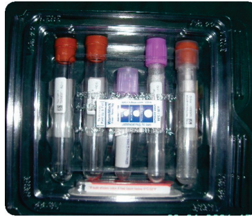
Exhibit 2-1. Placement of threshold temperature monitors in the refrigerated clamshell
