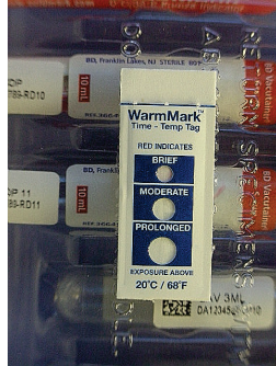
Exhibit 2-4. Triggered upper threshold temperature monitor
