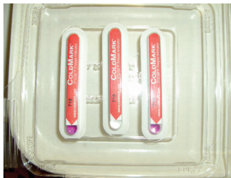
Exhibit 2-11. Lower threshold temperature monitor
