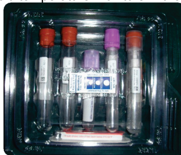
Exhibit 2-12. Placement of threshold temperature monitors in the refrigerated clamshell
