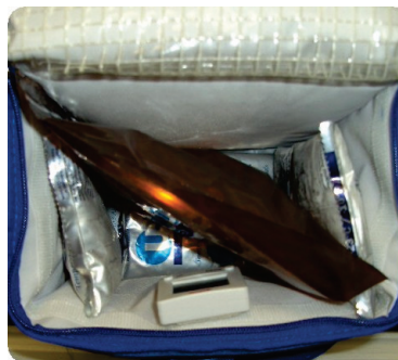
Exhibit 2-2. Proper packing of the refrigerated chamber
