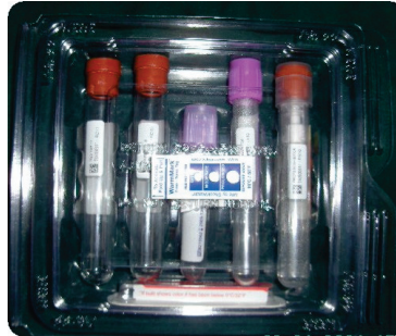
Exhibit 2-6. Placement of threshold temperature monitors in the refrigerated clamshell
