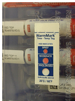
Exhibit 2-10. Triggered upper threshold temperature monitor
