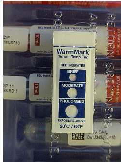
Exhibit 2-14. Triggered upper threshold temperature monitor
