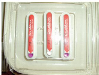
Exhibit 2-5. Lower threshold temperature monitor
