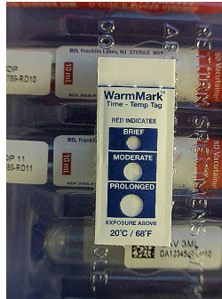
Exhibit 2-10. Triggered upper threshold temperature monitor
