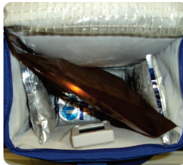
Exhibit 2-7. Proper packing of the refrigerated chamber
