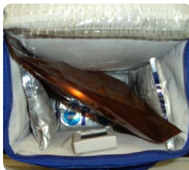
Exhibit 7-2. Proper packing of the refrigerated chamber
